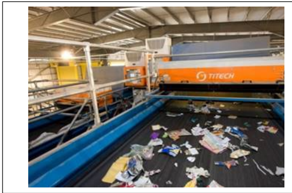
Figures 6, 7 and 8 Mechanical and manual sorting is used to separate different waste types for recycling at the MRF
