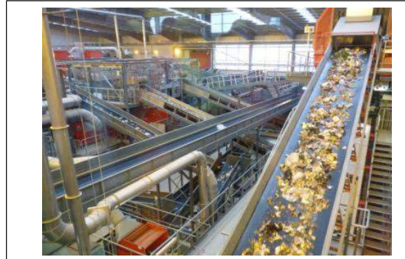
Figure 10 Shredded waste is sorted on conveyors
