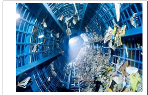
Figures 6, 7 and 8 Mechanical and manual sorting is used to separate different waste types for recycling at the MRF
